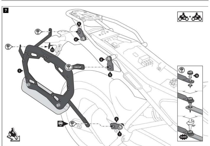
$\triangle$  **NOTE:** The SW-MOTECH anti-theft protection devices are available separately; mount the anti-theft protection devices on both sides at the indicated position. a
