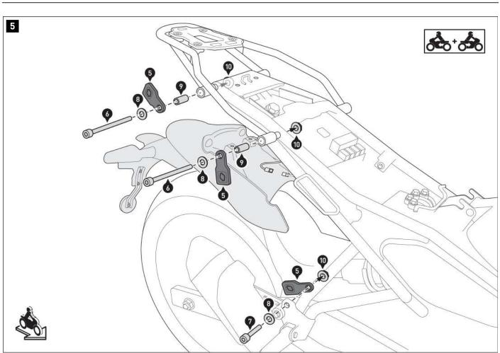
Screw the fastening tabs (5) **onto both sides** of the passenger grab handles and passenger footrest holders. Do not tighten the screws (6) and (7) yet.
