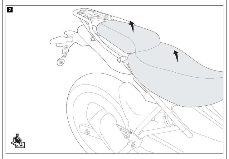
Remove the passenger seat and seat from the vehicle.
