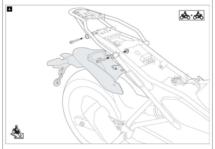
Remove the screws and nuts of the passenger grab handles  ${\bf on\;both\;sides}$  .
