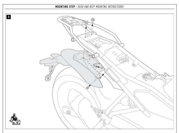
Loosen the four screws on the fender; then disconnect the fender connector.
