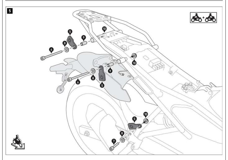
Screw the fastening tabs (5) **onto both sides** of the passenger grab handles and passenger footrest holders.
