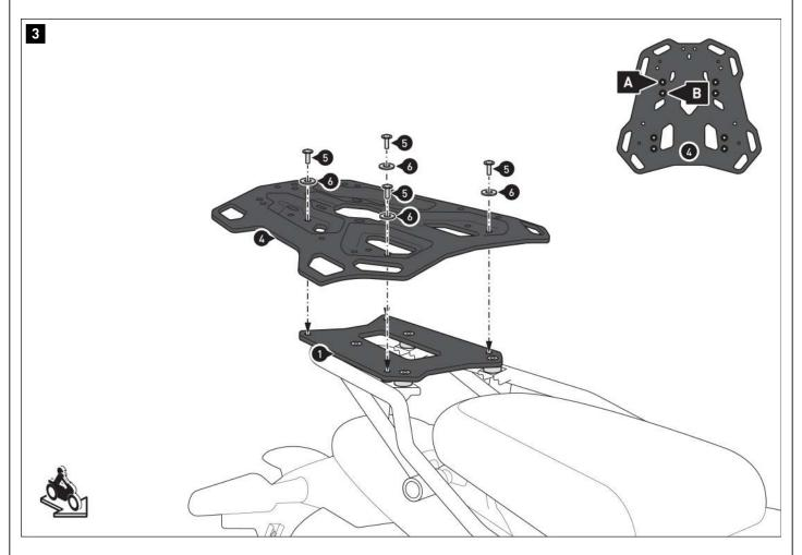
$\triangle$  **NOTE:** Depending on the space available, screw the luggage carrier (4) to the marked attachment position (A) or (B) as shown in the detailed drawing.
