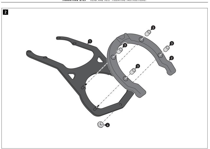
Insert the vibration dampener (4) into the indicated opening in the mounting bracket (1).
