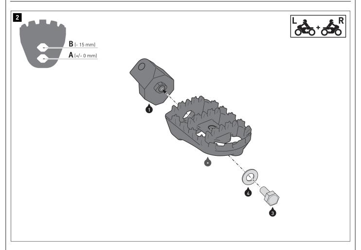
$\triangle$  **NOTE:** The indicated part (\*) is included with SW-MOTECH ION footrests (FRS.00.011.1000\*/\*).
