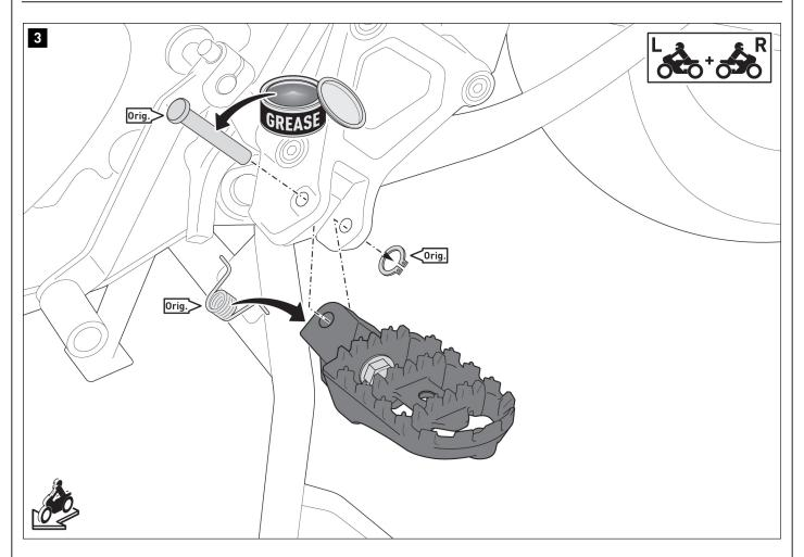
Install the joint adapters (1/2) using the original parts (0rig.) on both sides of the vehicle.
