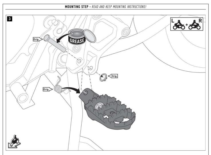
Clean the footrest mounts thoroughly. Apply rolling bearing grease to the original bolts (Orig.).
