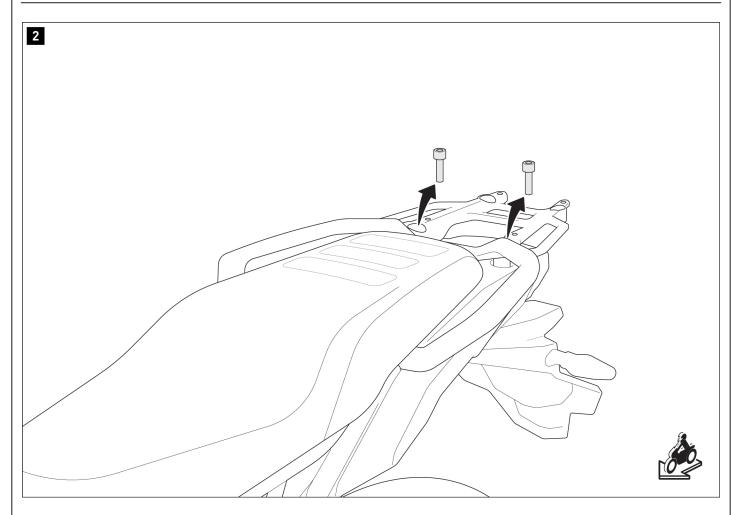
Remove the original screws from the rack.
