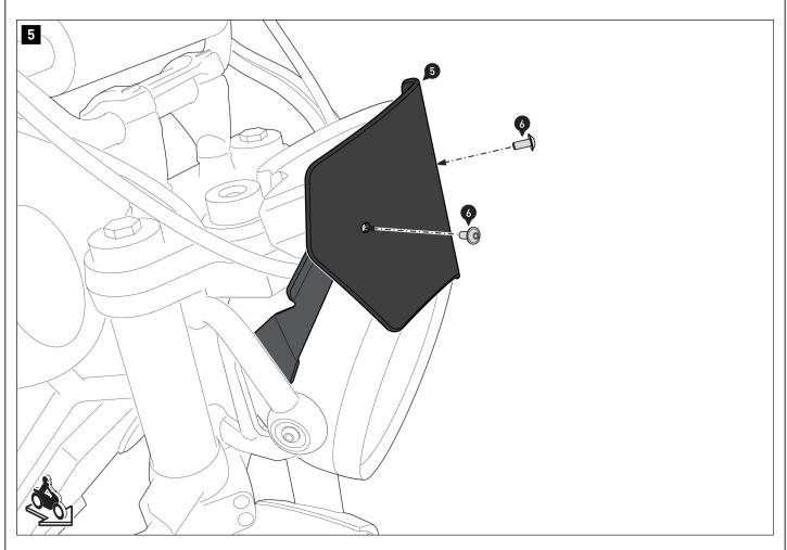
Screw the windscreen (5) to the mounting brackets (1) and (2). **A WARNING: Use liquid threadlocker!** Tighten the screws (6) as specified.
