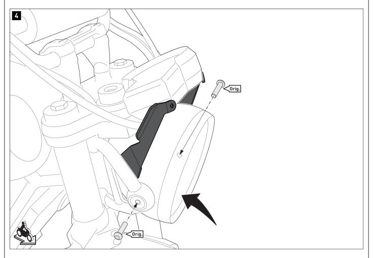
Reinstall the original headlight on the vehicle. **A ATTENTION:** Make sure that the headlight is correctly adjusted!
