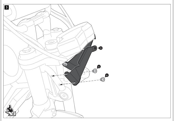
Screw the mounting bracket [3] to the vehicle. **AWARNING:** Use a liquid threadlocker!
