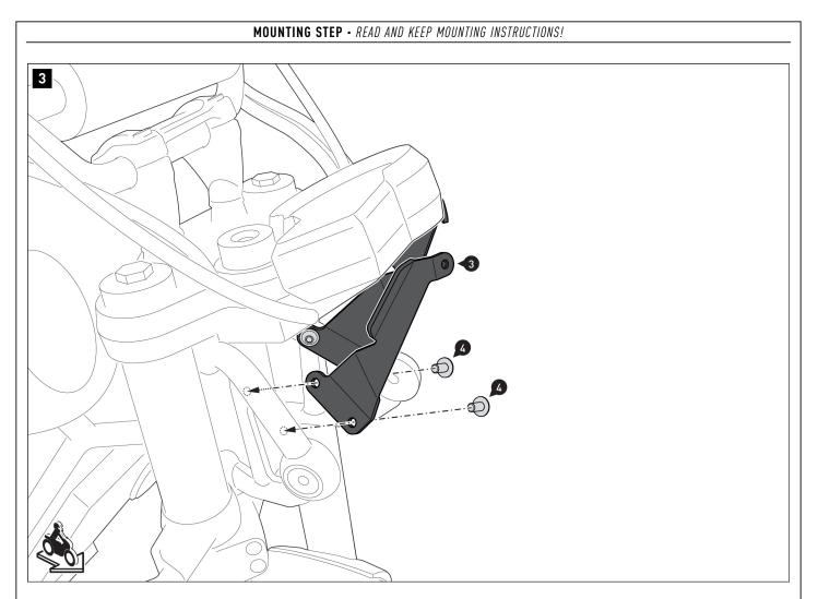
Screw the mounting bracket (3) to the vehicle. **AWARNING: Use a liquid threadlocker!** Tighten the screws (4) according to the vehicle manufacturer's specifications.
