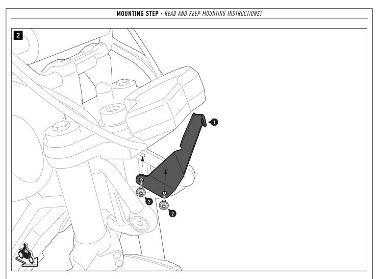
Screw the mounting bracket (1) to the vehicle. **AWARNING: Use a liquid threadlocker!** Tighten the screws (2) according to the vehicle manufacturer's specifications.
