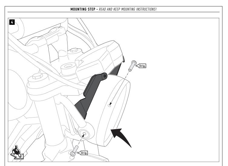
Reinstall the original headlight on the vehicle. ATTENTION: Make sure that the headlight is correctly adjusted!
