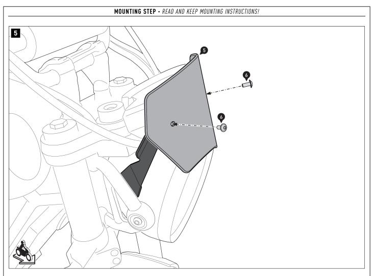
Screw the windscreen (5) to the mounting brackets (1) and (2). **A WARNING: Use liquid threadlocker**! Tighten the screws (6) as specified.
