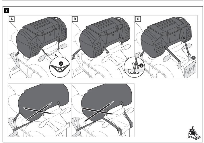
$\triangle$  **NOTE:** SW-MOTECH recommends attaching heavy-duty license plate holders to the lashing eyes (\*), which are available separately. Screw the lashing eyes (\*) behind the license plate using the original screws.
