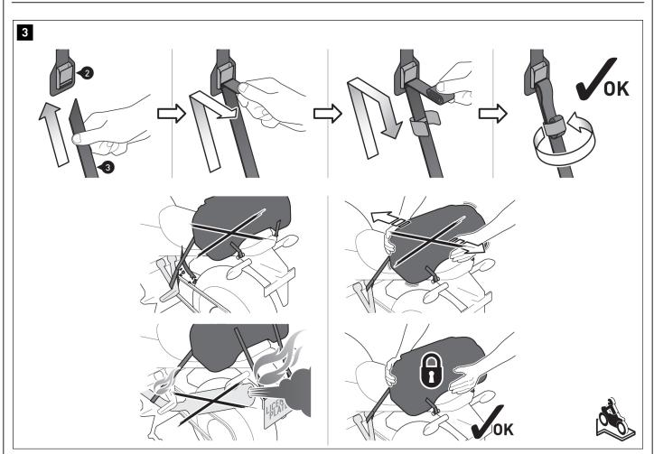
Pull the fastening straps (3) through the buckles of the tail bag (2). Now pull it tight until the tail bag (2) is centred and firmly attached to the vehicle.
