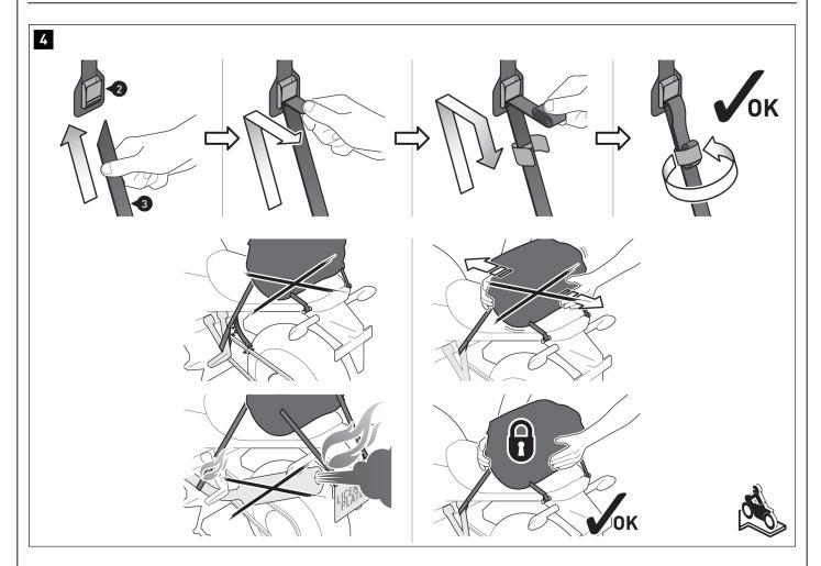
Pull the fastening straps (3) through the buckles of the tail bag (2). Now pull it tight until the tail bag (2) is centered and firmly attached to the vehicle.
