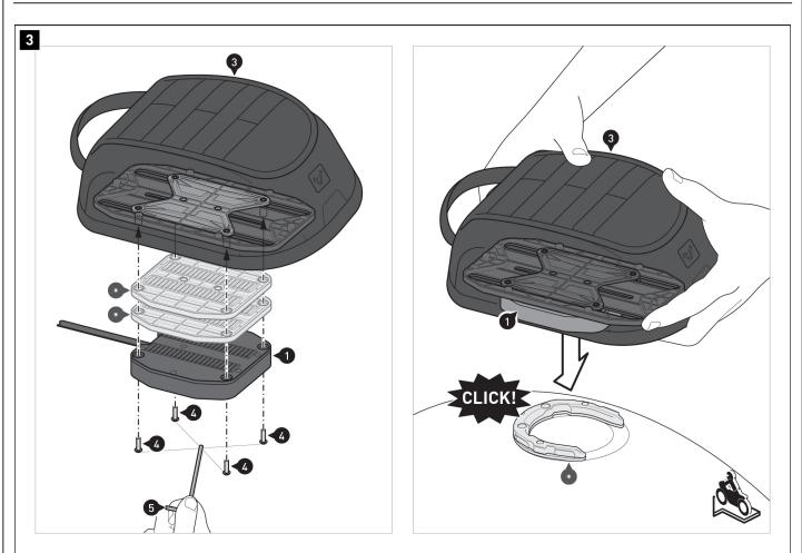
▲ NOTE: Some tank models require a height increasing element (sold separately) (\*).TRT.00.787.1010\* for additional 6 mm. TRT.00.787.1020\* for additional 12 mm. In the latter case, screws (4) are not required; instead, attach using the screws provided with the height increasing element (\*).
