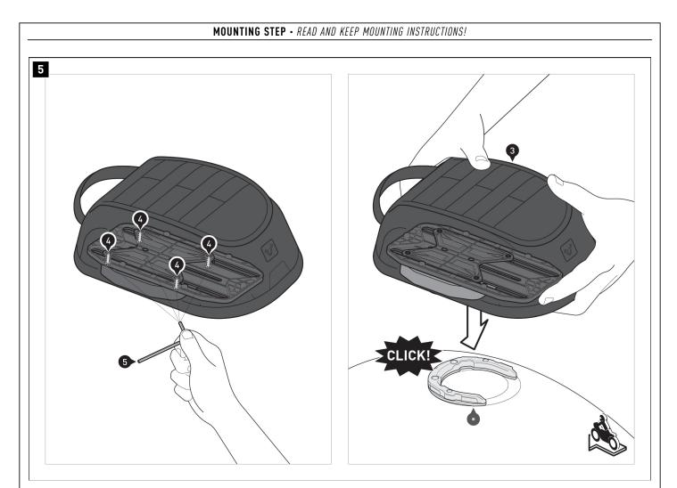
Now tighten the screws [4] as specified in the mounting instructions. **A** WARNING: Over-tightening the screws will damage plastic parts!
