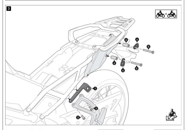
Screw fastening lugs (1/2) and (4) **onto both sides** of the bike. **A WARNING:** Use a liquid threadlocker! Do not tighten the screws (3) and (5) yet.
