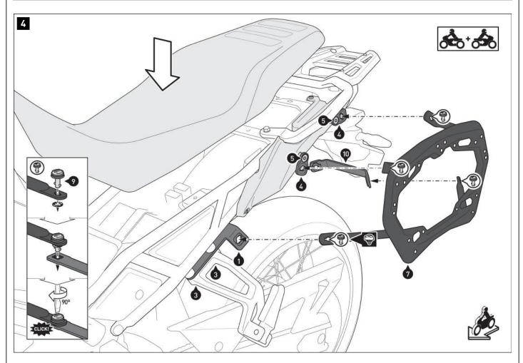
Connect the side supports (7/8) **on both sides** with the quick-release fasteners (9) on fastening lugs (1/2) and (4) as well as the cross connector (10). Secure the quick-release fasteners using the lock washers.
