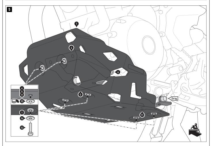
Use some grease to secure the washers (15) to the mounting brackets (4), (5) and (11).
