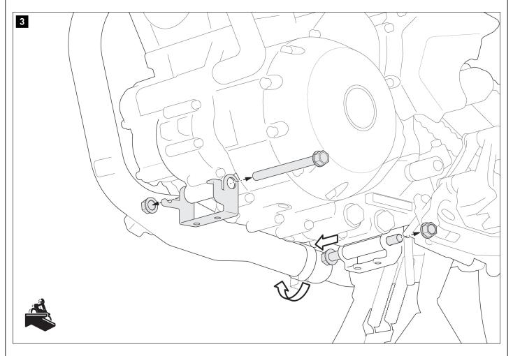
Loosen the nut on the front mounting bracket and remove it from the vehicle.
