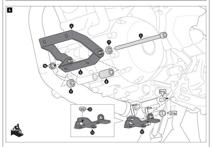
Screw the front mounting brackets (4) (external) and (5) (internal) onto the
