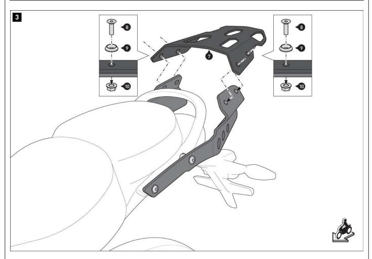
Screw the luggage rack (7) onto mounting brackets (1) and (2).
