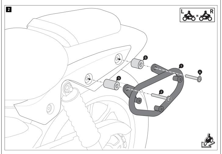
Screw the side carrier [1] to the rear of the vehicle. **A** WARNING: Use liquid threadlocker!
