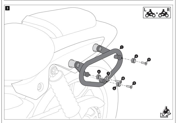
Screw parts (6) to (9) onto the side carrier (1). **A** WARNING: Use liquid threadlocker!
