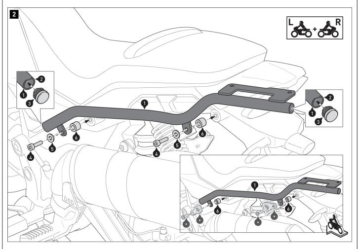
⚠ NOTE: If installing at the same time as the SW-MOTECH carrier (\*), screw the parts together as shown in the detailed drawing. The screws (4) and washers (5) are no longer required. Instead, mount the screws (\*) included with the carrier.
