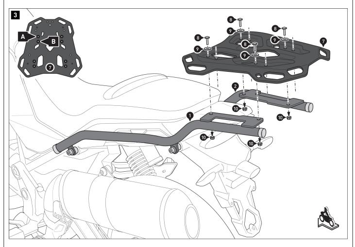
$\triangle$  **NOTE:** Depending on the space available, screw the rack (7) to the marked mounting position **(A)** or **(B)** as shown in the detailed drawing.
