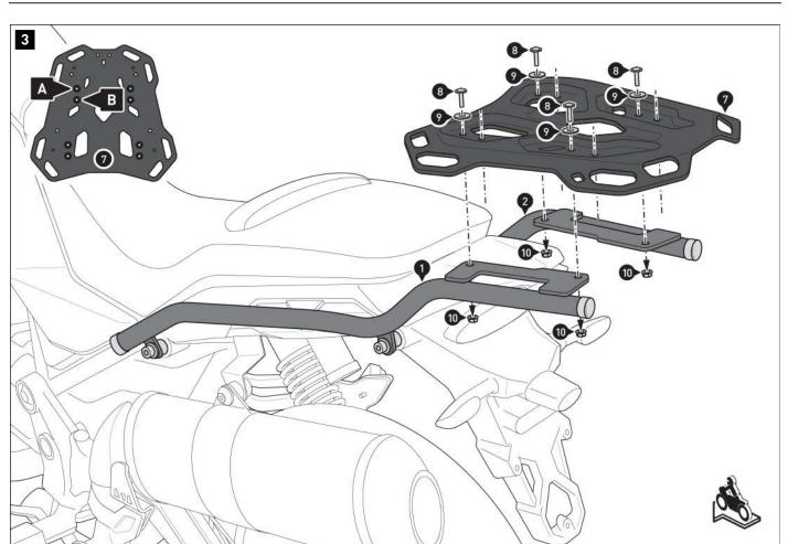
**NOTE:** Depending on the space available, screw the rack (7) to the marked mounting position(A) or(B) as shown in the detailed drawing.
