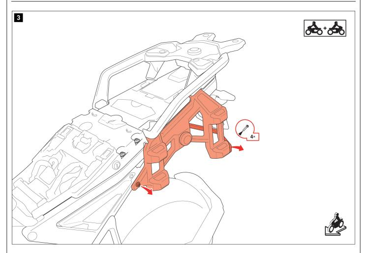
Loosen the marked screws  $\mbox{\bf on both sides}$  (2x per vehicle side) and remove the crossbar from the vehicle.
