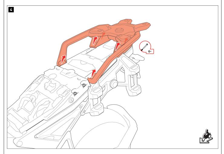
Loosen the marked screws  $\mbox{\bf on both sides}$  (3x per vehicle side) of the original rack.
