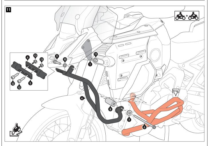
Screw the crash bar halves (4/5) on both sides to the mounting brackets (1/2) and the original crash bars (0rig.]).
