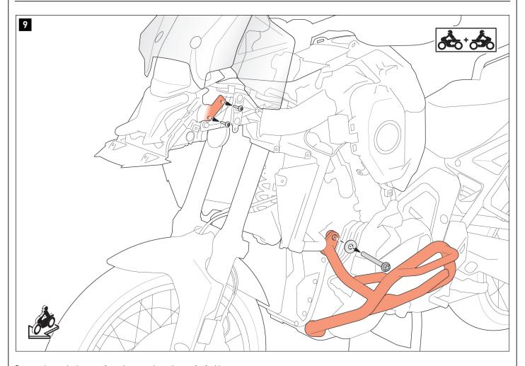
Remove the marked screws from the mounting points on **both** sides.  $\triangle$  **NOTE:** Make sure that the internal spacers on the original crash bar stay in place.
