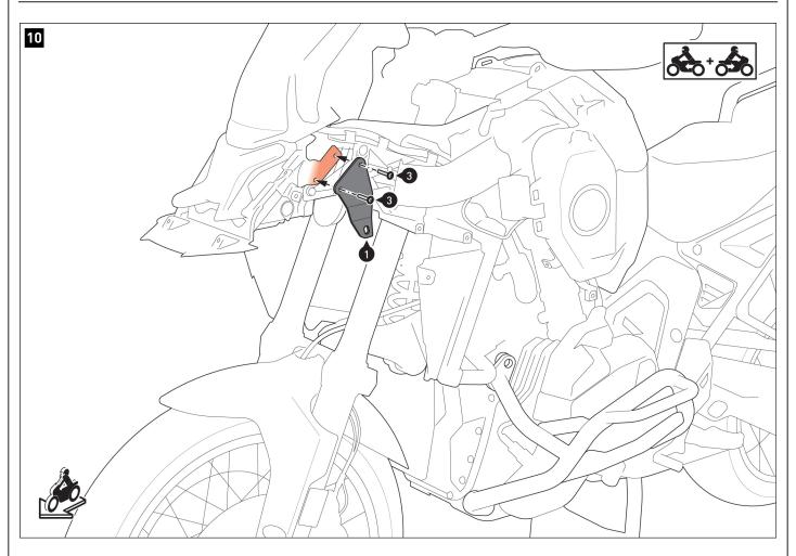
Screw the mounting brackets (1/2) **onto both sides** of the vehicle. **A WARNING:** Use a liquid threadlocker! Tighten the screws (3) according to the vehicle manufacturer's specifications.
