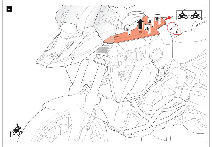
Loosen the marked screws **on both sides** (1x per vehicle side) and remove the fairings from the vehicle. **\tilde{\Delta} NOTE:** Pay attention to the marked plug anchors on the fairings.
