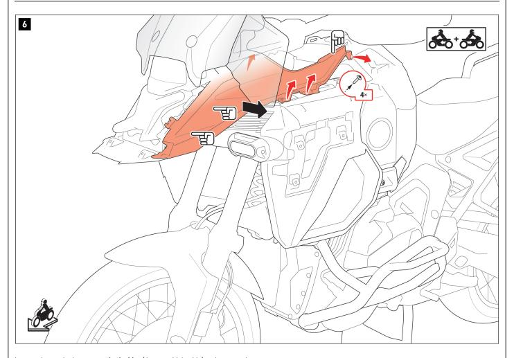
Loosen the marked screws **on both sides** (4x per vehicle side) and remove the fairing from the vehicle. **\tilde{\Delta} NOTE:** Pay attention to the marked plug anchors on the fairings.
