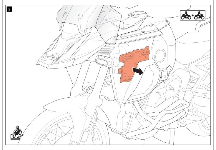
Remove the inner fairings from  ${\bf both\ sides}$  of the vehicle.
