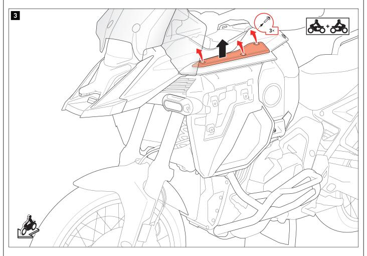
Loosen the marked screws  ${\bf on\ both\ sides}$  (3x per vehicle side) and remove the fairings from the vehicle.
