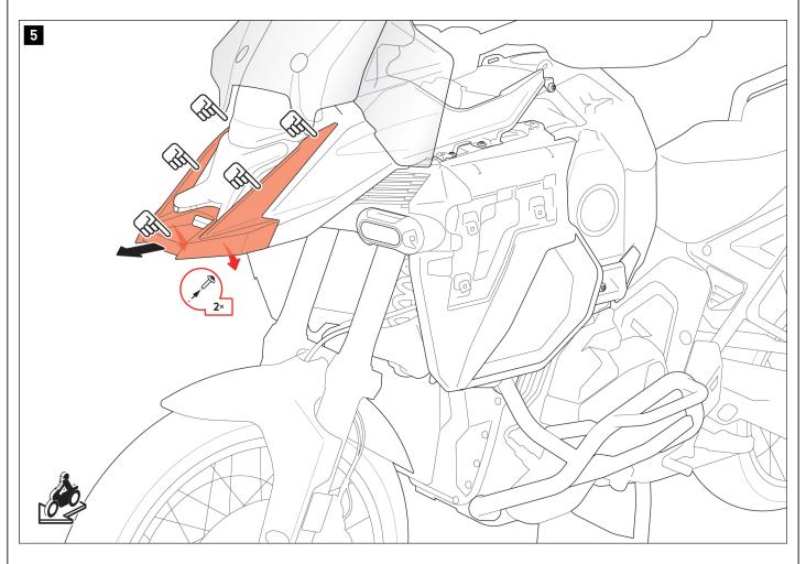
Loosen the marked screws (2x) and remove the fairing from the vehicle.  $\triangle$  **NOTE:** Pay attention to the marked plug anchors on the fairing.
