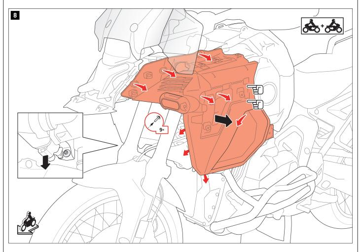
$\triangle$  **NOTE:** On the **right** side of the vehicle, the plug shown in the detailed drawing must first be pulled out of its anchorage.
