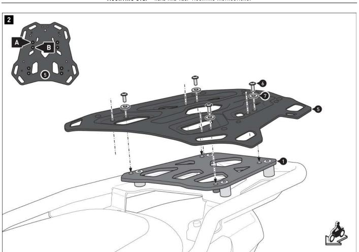
▲ **NOTE:** Depending on the space available, screw the luggage carrier (5) to the marked mounting position (A) or (B) as shown in the detailed drawing.
