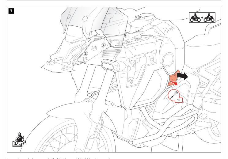
Loosen the marked screws **on both sides** (1x per vehicle side) and remove the fairings from the vehicle. **\tilde{\Delta} NOTE:** The fairings are secured by two plug connections.
