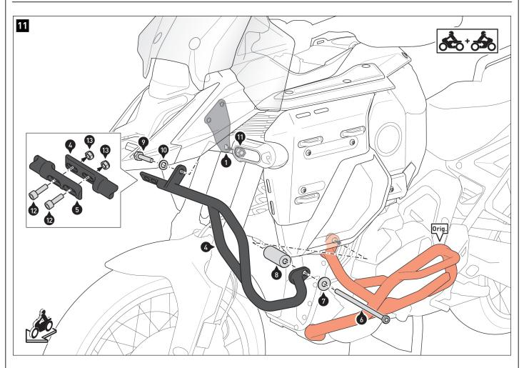
Screw the crash bar halves [4/5] on both sides to the mounting brackets [1/2]
