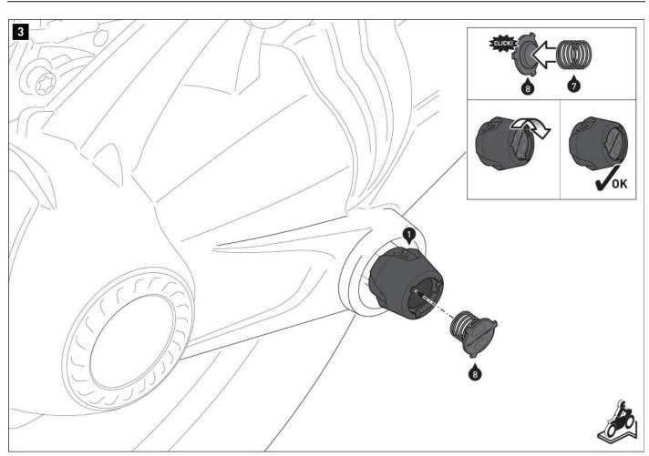
Insert the spring (7) into the cover cap (8) as shown in the detailed drawing.
