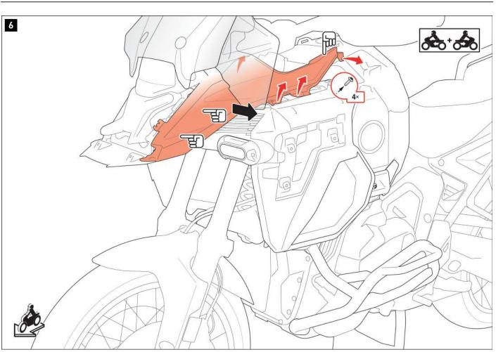
Loosen the marked screws **on both sides** (4x per vehicle side) and remove the fairing from the vehicle. *NOTE:* Pay attention to the marked plug anchors on the fairings.
