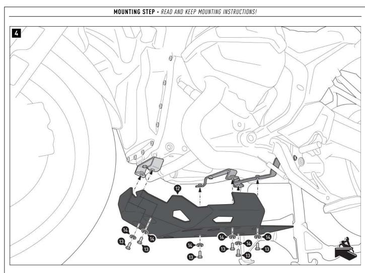
Screw the engine guard (12) onto the mounting brackets (1), (2) and (3). **A WARNING: Use a liquid threadlocker!** Tighten the screws (13) as specified in the mounting instructions.
