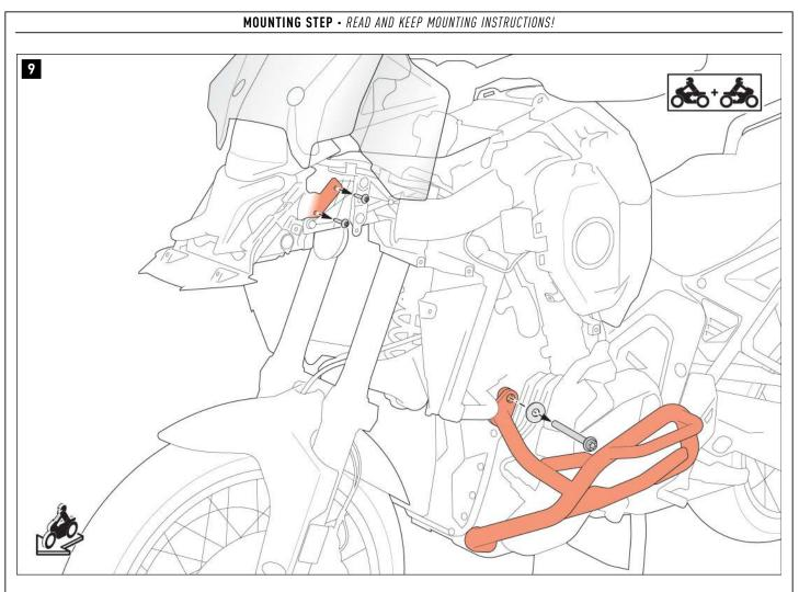
Remove the marked screws from the mounting points on **both** sides. *NOTE:* Make sure that the internal spacers on the original crash bar stay in place.
