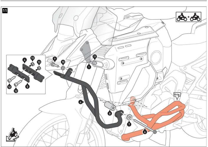
Screw the crash bar halves (4/5) **on both sides** to the mounting brackets (1/2) and the original crash bars (Orig.)). **A** WARNING: Use liquid thread locker (screws (6) only)! Do not tighten screws (6) and (9) yet.
