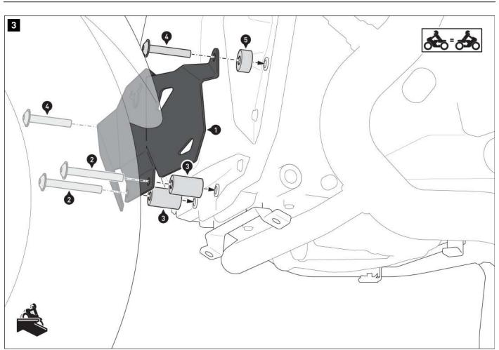
Screw the engine guard extension (1) onto the vehicle. **A WARNING: Use a liquid threadlocker!** Tighten the screws (2) and (4) according to the manufacturer's instructions.
