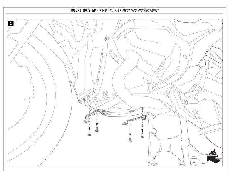
Remove the original retaining plates from the vehicle.
