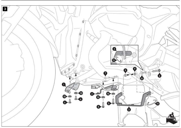
Screw the front (1), middle (2) and (3) rear mounting brackets to the vehicle. **A WARNING: Use liquid thread locker (only for screws (4) and (5))!** Tighten the screws (4) and (5) according to the vehicle manufacturer's specifications. Tighten the screws (6) and (7) as specified in the mounting instructions.
