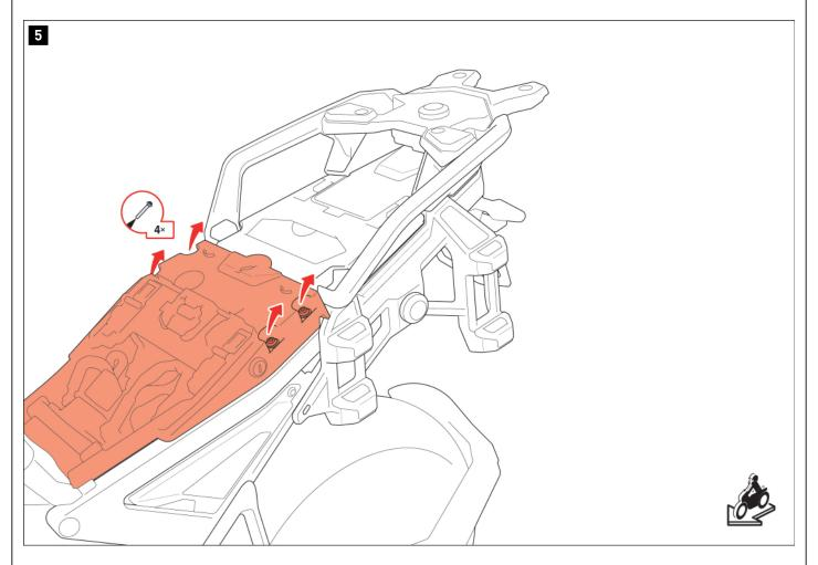
Loosen the marked screws  $\mbox{\bf on both sides}$  (2x per vehicle side) of the frame cover.
