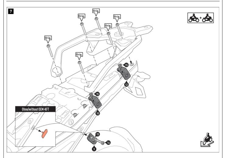
$\triangle$  **NOTE:** Pay attention to the hole spacing of the mounting brackets (10/11) and (12/13); the mounting brackets (10/11) with the smaller hole spacing are mounted at the front in the direction of travel, the mounting brackets (12/13) with the larger hole spacing are mounted at the rear in the direction of travel.
