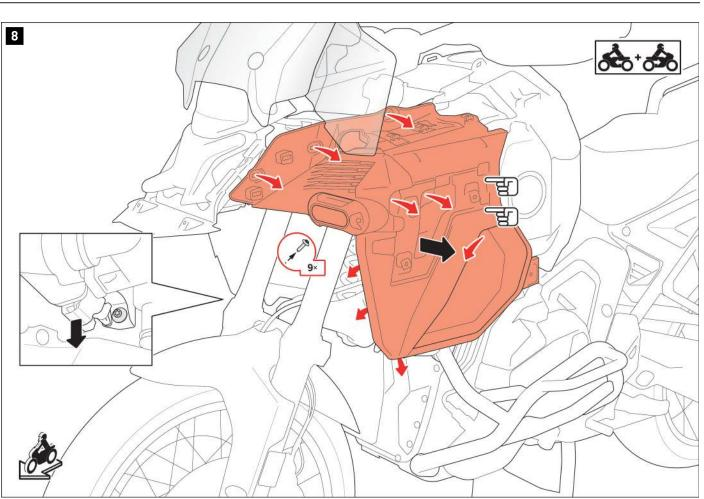
**NOTE:** On the **right** side of the vehicle, the plug shown in the detailed drawing must first be pulled out of its anchorage.
