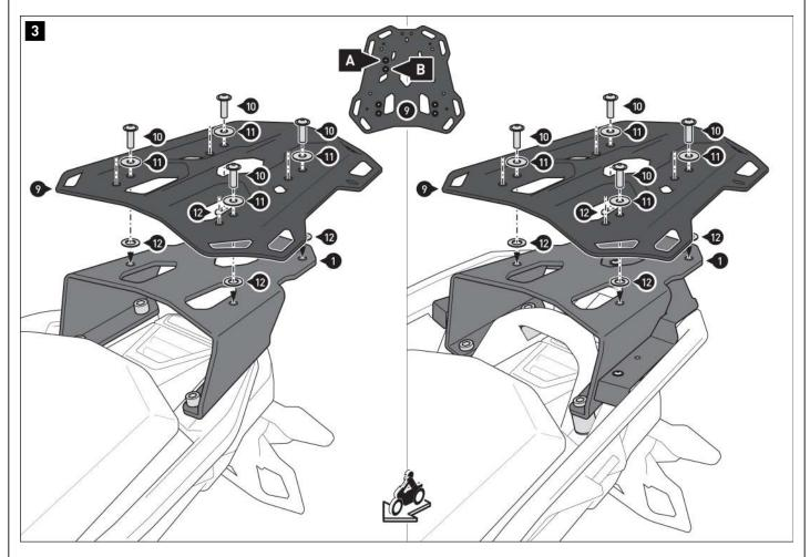
$\triangle$  NOTE: Depending on the space available, screw the rack to the marked mounting position (A) or (B) , as shown in the detailed drawing .
