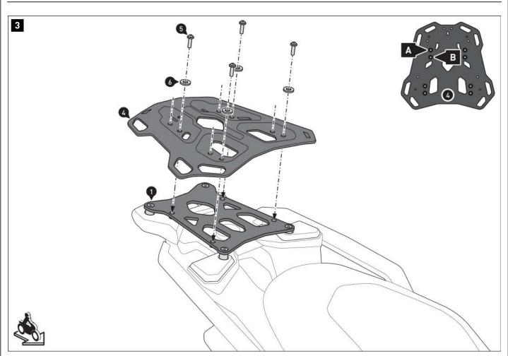
▲ **NOTE:** Depending on the space available, screw the rack (4) to **mounting position (A)** or **(B)**, as shown in the detailed drawing.
