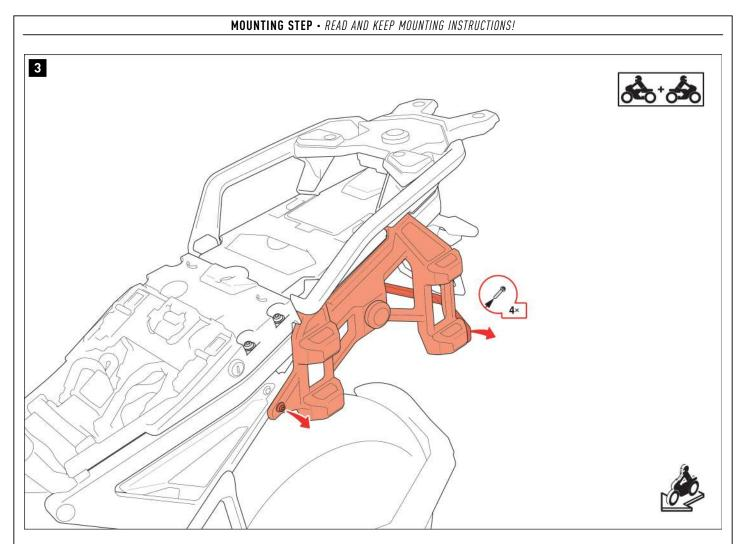
Loosen the marked screws  ${\bf on \ both \ sides}$  (2x per vehicle side) and remove the crossbar from the vehicle.
