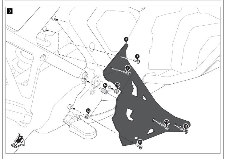
Screw the heel guard onto the **right** side of the vehicle. **A WARNING:** Use a liquid threadlocker! Tighten screws [9], [10], [11] and [12] according to the vehicle manufacturer's specifications.
