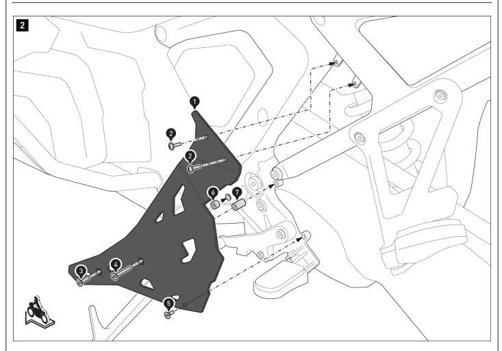
Screw the heel guard onto the **left** side of the vehicle. **A** WARNING: Use a liquid threadlocker!
