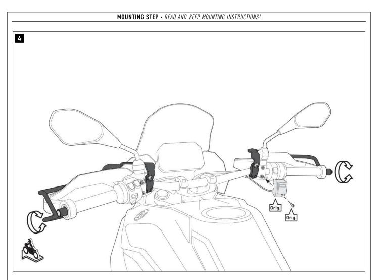
Align the hand protector so that it does not come into contact with the windshield when the steering is fully turned.
