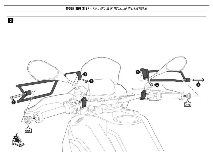
Screw the two hand protectors (2) and (3) to the original handlebar ends (orig.) on the vehicle. **A WARNING: Use a liquid threadlocker!** Do not tighten screws (4) and (5) yet.
