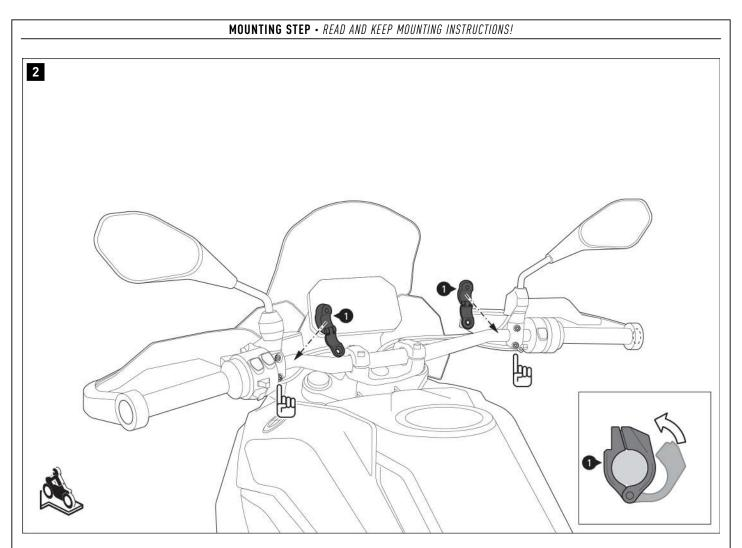
Place the two clamps (1) around the handlebars.
