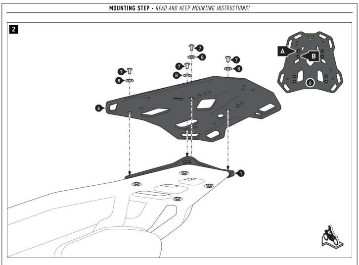
▲ **NOTE:** Depending on the space available, screw the rack (6) to the marked mounting position (A) or(B) as shown in the detailed drawing.
