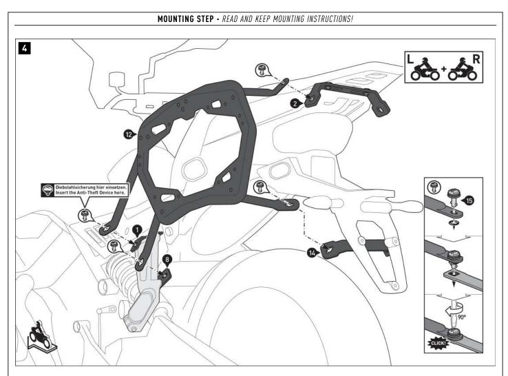
**NOTE:** SW-MOTECH anti-theft protection is sold separately; mount the anti-theft protection devices on both sides at the marked position.
