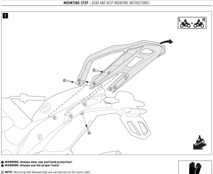
Unscrew the screws from  ${\bf both\ sides}$  of the original rack and remove it from the vehicle.
