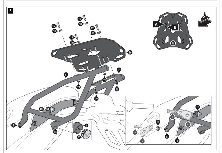
$\bigtriangleup$  NOTE: Screws (3) and (9) are not required if mounting the SW-MOTECH side
