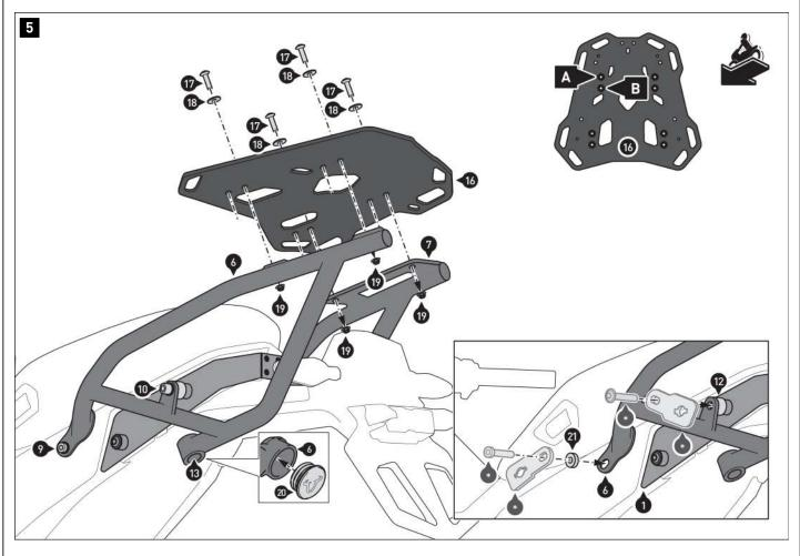
riangle **NOTE:** Screws (3) and (9) are not required if mounting the SW-MOTECH side
