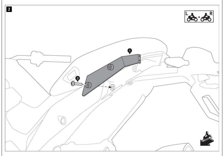
Mount the cover plates [1/2] onto both sides of the vehicle. **A WARNING:** Use liquid thread locker.
