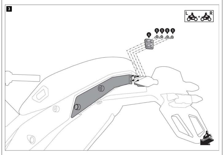
Connect the cover plates (1/2) to the connecting plate (4). **A** WARNING: Use liquid thread locker.
