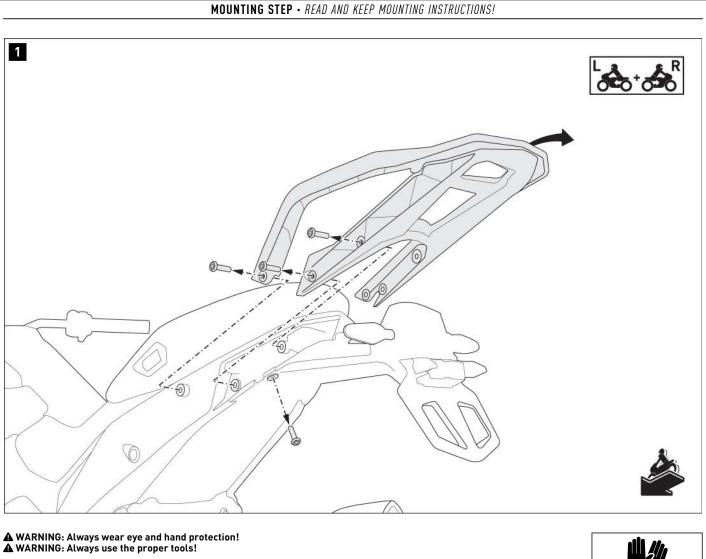
▲ NOTE: Mounting and disassembly are carried out on the same side!
