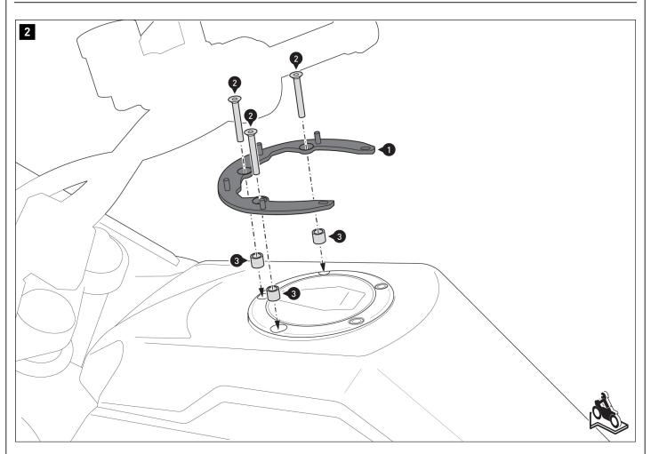
Screw the mounting ring (1) onto the vehicle. **A** WARNING: Use a liquid threadlocker!
