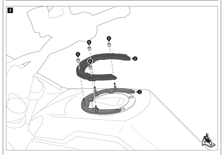
Carefully screw the tank ring (4) onto the mounting ring (1).
