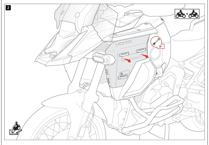
Remove the marked screws  ${f on\ both\ sides}$  (2 per vehicle side).
