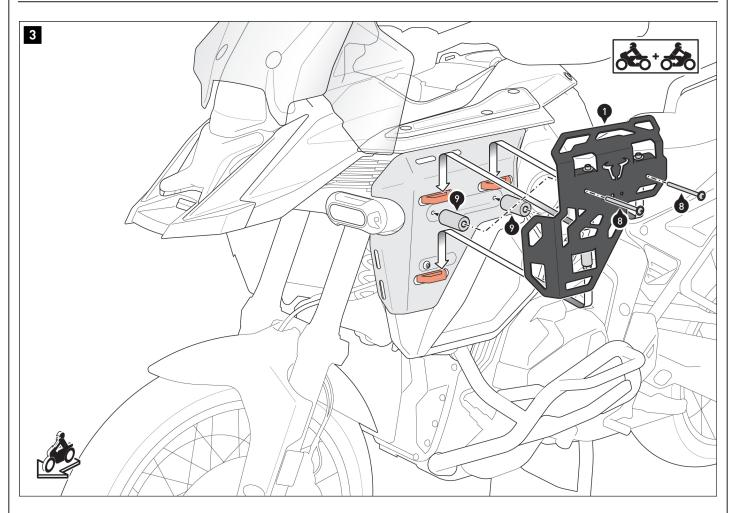
Hang the support plates (1/2) with the spacer (5) on  $\bf both\ sides$  of the three luggage holding points of the bike.
