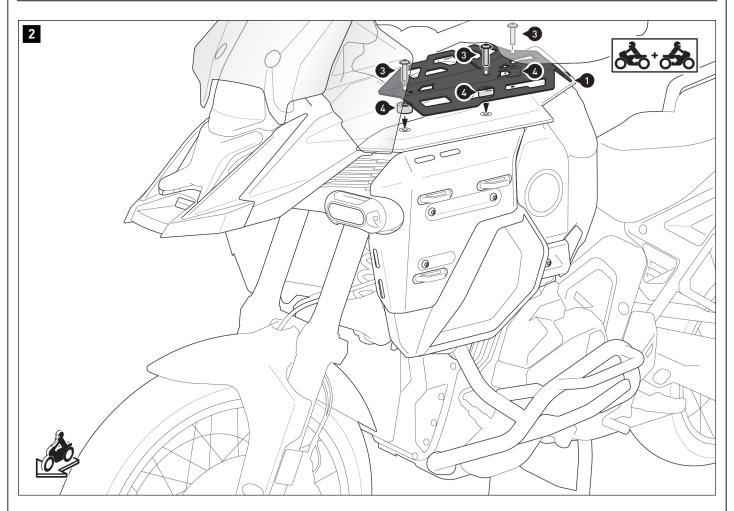
Screw the tank shelves (1/2) **onto both sides** of the bike. **A WARNING:** Use a liquid threadlocker! Tighten the screws (3) according to the vehicle manufacturer's specifications.
