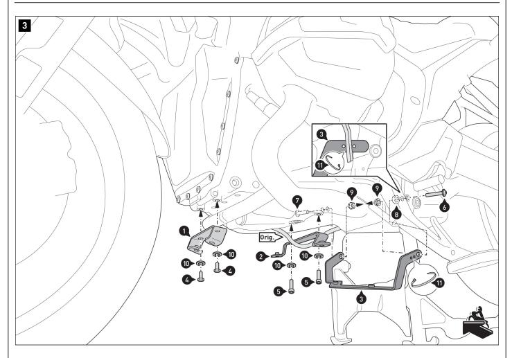
Screw the front (1), middle (2) and (3) rear mounting brackets to the vehicle.
