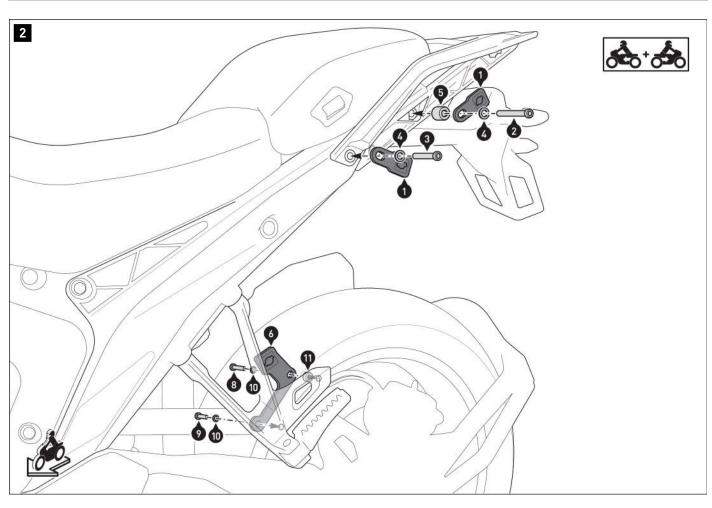
Screw in the fastening straps (1), (6), and (7) on both sides of the vehicle. **A WARNING: Use a liquid threadlocker!** Do not tighten the screws (2), (3), (8) and (9) yet.
