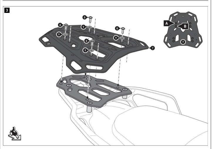
**△ NOTE:** Depending on the space available, screw the luggage carrier (7) to the marked mounting position (A) or (B) as shown in the detailed drawing.
