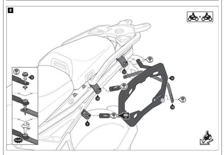
Assemble all parts described in steps  $\[1\]$  to  $\[6\]$  dismantled original parts back on the vehicle in reverse order.
