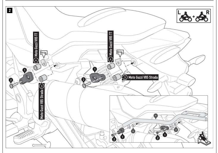
$\triangle$  **NOTE:** The parts of the OEM luggage rack (Orig.) of the vehicle model V85 TT shown are schematic and are intended only as a guide during installation.
