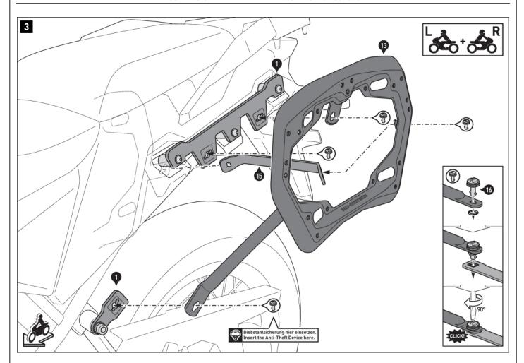
Connect the side carriers (13) and (14) with the quick-release fasteners (16) to the mounting brackets (1) and (5) and crossbar (15). Secure the quick-release fasteners using the lock washers.
