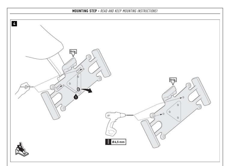
Use a suitable tool to mark the two drilling points on the back of the license plate holder (Orig.). Then loosen the screw (4) and remove the license plate holder from the
