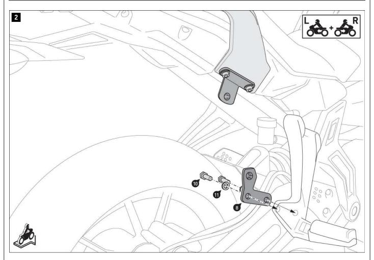
Screw the mounting brackets (8) and (9) on both sides of the vehicle behind the passenger footrests.
