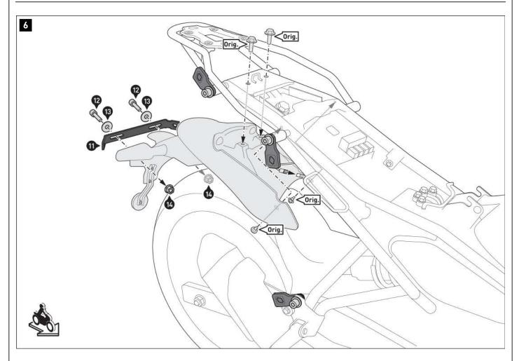
Screw the cross connector (11) to the license plate holder of the fender. Do not tighten the screws (12) yet.
