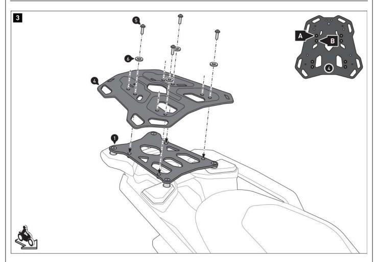
$\triangle$  **NOTE:** Depending on the space available, screw the rack (4) to **mounting position (A)** or **(B)**, as shown in the detailed drawing.
